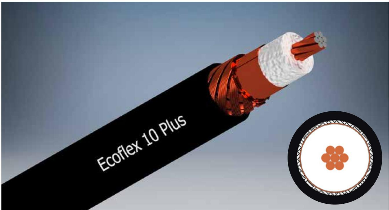
Ecoflex 10 Plus is an extremely flexible, low loss coaxial cable designed to use in the frequency range up to 8 GHz. Advanced manufacturing techniques combined with the use of a low loss PE-LLC dielectric with a foaming rate of more than 70% result in very low attenuation values, which set standards among flexible coaxial cables.
