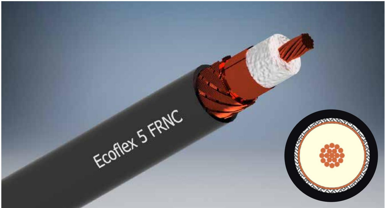
Ecoflex 5 FRNC is a thin and extremely flexible coaxial cable designed for frequencies up to 6 GHz. Due to its low loss in relation to the outer diameter of 5,5 mm and the very small bending radius the cable can be used for numerous RF applications.
