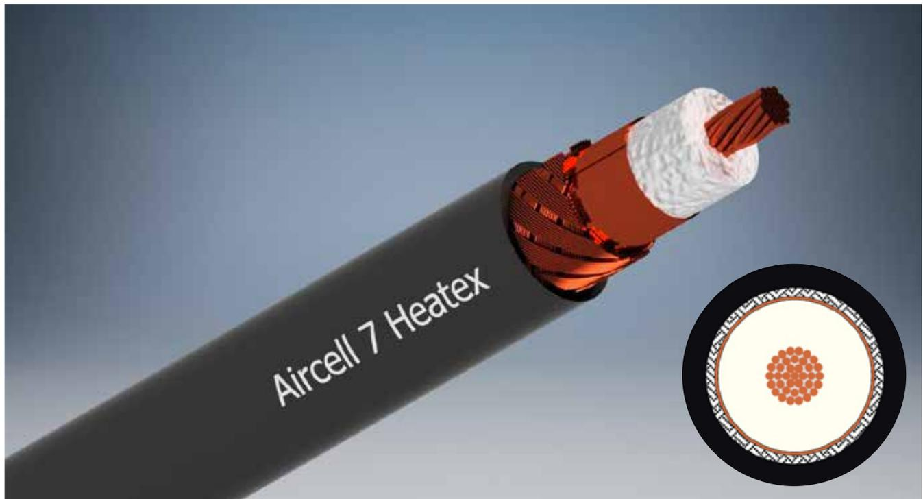
Aircell 7 Heatex is an ultraflexible coaxial cable designed for frequencies up to 6 GHz. Due to its low loss in relation to the outer diameter and the small bending radius the cable can be used for numerous RF applications.
