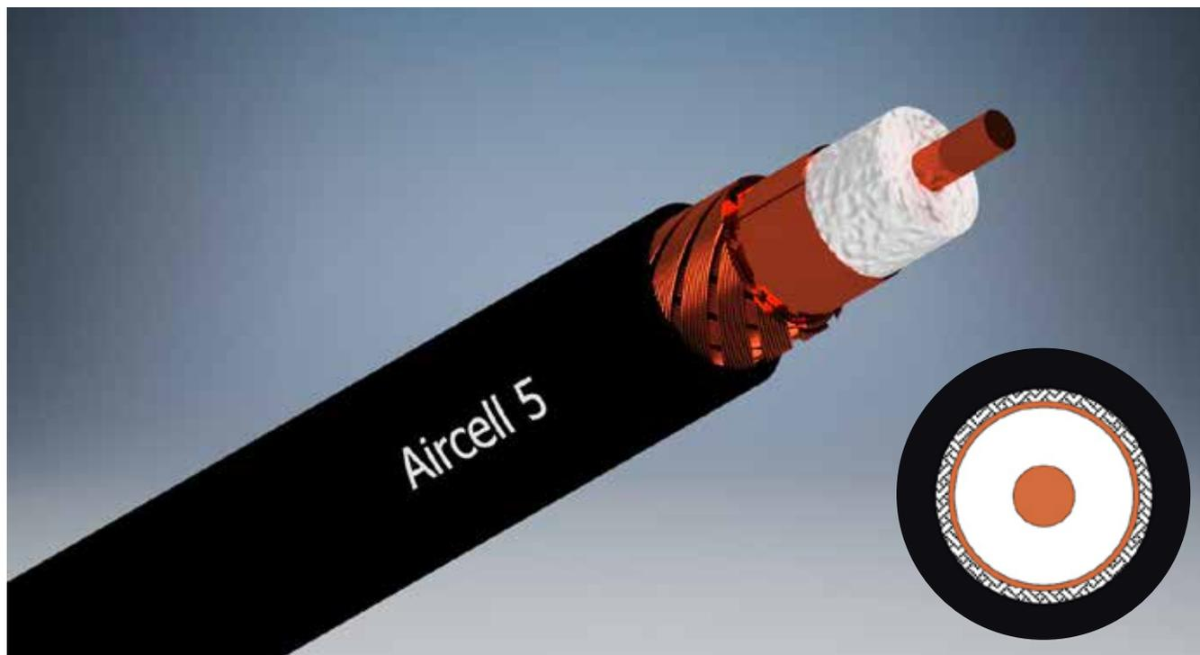
Aircell 5 is a flexible and thin coaxial cable with 5 mm outer diameter for the frequency range from DC to 10 GHz. Its low loss characteristics in relation to the diameter and the ability to use standard RG 58 connectors make this cable the number one choice not only for Wireless LAN applications but also for general RF communications.
