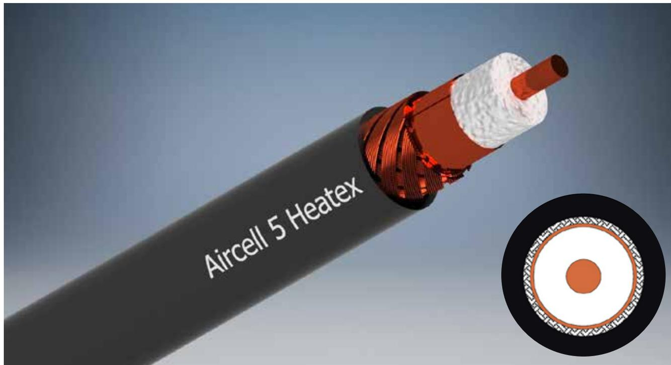
Aircell 5 Heatex is a flexible and thin coaxial cable with 5 mm outer diameter for the frequency range from DC to 10 GHz. Its low loss characteristics in relation to the diameter and the ability to use standard RG 58 connectors make this cable the number one choice not only for Wireless LAN applications but also for general RF communications.
