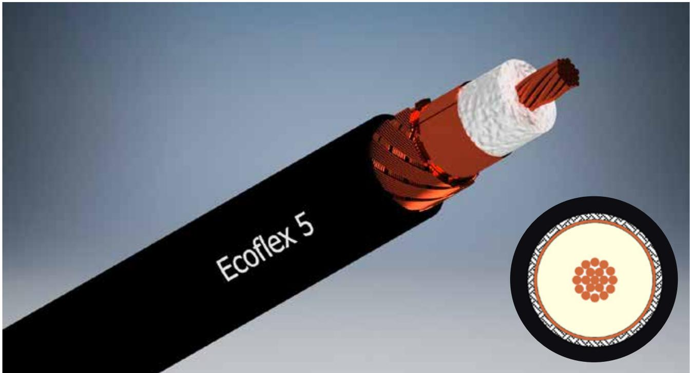
Ecoflex 5 is a thin and extremely flexible coaxial cable designed for frequencies up to 6 GHz. Due to its low loss in relation to the outer diameter of 5,5 mm and the very small bending radius the cable can be used for numerous RF applications.
