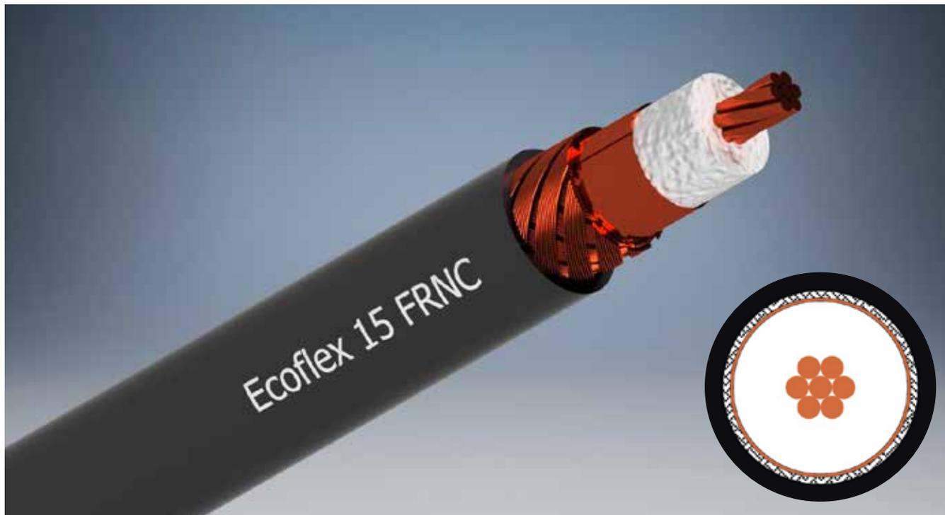
Ecoflex 15 FRNC is a flexible low loss 50 ohm coaxial cable for the frequency range up to 6 GHz. Advanced manufacturing techniques combined with the use of a low loss PE-LLC dielectric with a foaming rate of more than 70% result in very low attenuation values.
