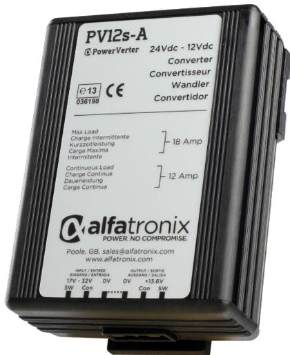
Alfatronix have developed three voltage converters, a 3Amp, 6Amp (continuous) and a 12A (continuous), which overcome these configuration problems. The Alfatronix converters mimic the 12V battery and 12V ignition function by providing two outputs, either of which can provide full power. One output is available whenever the 24V battery is connected. The other output is switched by the 24V ignition switch. Now the ICE equipment can be fitted to the 24V truck as simply as fitting it to a 12V car.
