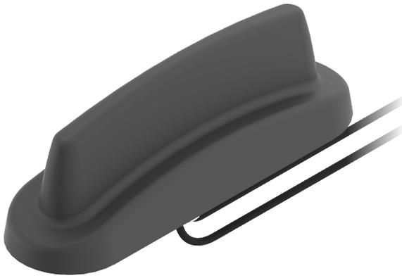
The LP[G]AM-BC3G-26-[XSP] range has been designed to provide MiMo Cellular /LTE antenna function for IOT and M2M applications. The compact, robust low-profile housing is weatherproof and contains two antenna elements with effective isolation and correlation covering all current global cellular and LTE bands in freq. range 698-960/1710-3800MHz. The LG version includes an active GPS/GNSS/Galileo/Beidou antenna for applications which require position or timing function.
