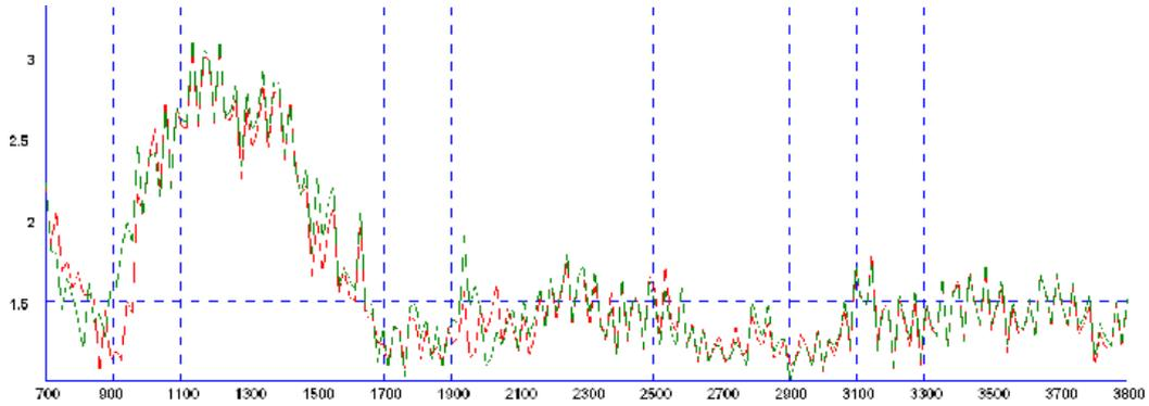
\*VSWR measured with 3m (10') of RG174 cable a) Red: in free space b) Green: on a 400x400mm (1'4") ground plane
