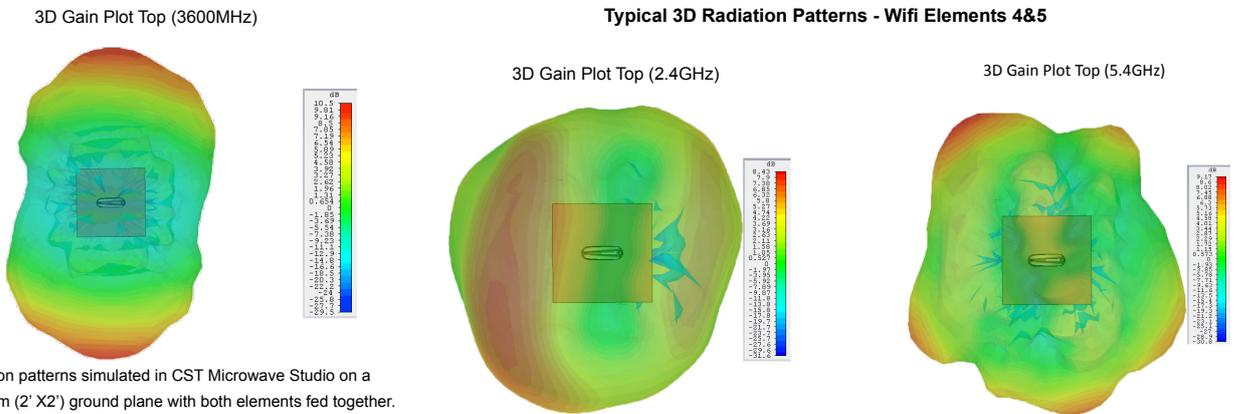
\*3D radiation patterns simulated in CST Microwave Studio on a 600x600mm (2' X2') ground plane with both elements fed together.
