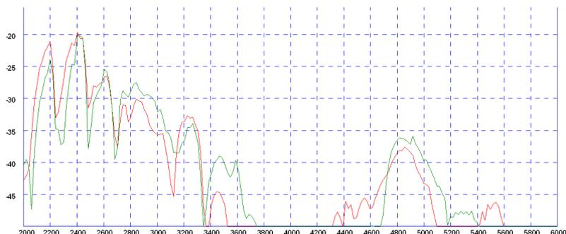
\*Isolation measured with 3m (10') of RG174 cable a) Red: in free space b) Green: on a 400x400mm (1'4") ground plane
