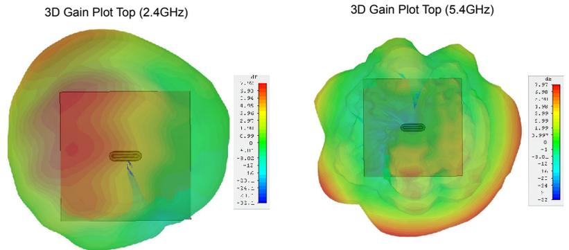
\*3D radiation patterns simulated in CST Microwave Studio on a 600x600mm (2' X2') ground plane with a single element feed.
