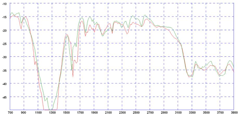
\*Isolation measured with 3m (10') of RG174 cable a) Red: in free space b) Green: on a 400x400mm (1'4") ground plane
