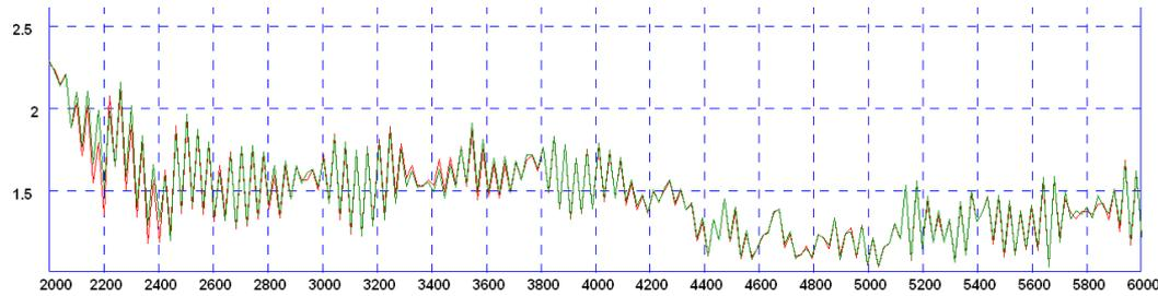
\*VSWR measured with 3m (10') of RG174 cable a) Red: in free space b) Green: on a 400x400mm (1'4") ground plane
