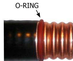
5. Install rear portion of connector over the O-ring, then pull forward so that the forward edge of the connector is covering the spring fingers and aligned over the corrugation peak.
