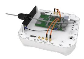
Carefully place the CPE back cover to close the CPE and screw the fasteners firmly. Do not over-tighten the screws, as this could strip the plastics.
