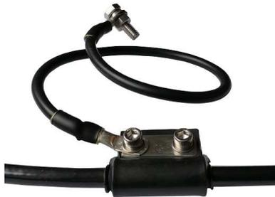
The GC-10 grounding clamp was developed for equipotential bonding on 10 mm coax cables such as ECOFLEX 10, Aircom Premium etc. This eliminates potential differences (voltages) between the coax cable and the earth potential. Especially during thunderstorms, charging can occur on the antenna or on the coax cable. This charge is removed with the earthing clamp and the connected device is protected. A grounding clamp is not a replacement for lightning protection.
