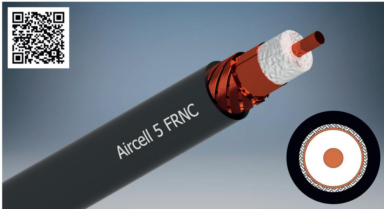
Aircell 5 FRNC is a flexible and thin coaxial cable with 5 mm outer diameter for the frequency range from DC to 10 GHz. Its low loss characteristics in relation to the diameter and the ability to use standard RG 58 connectors make this cable the number one choice not only for Wireless LAN applications but also for general RF communications.
