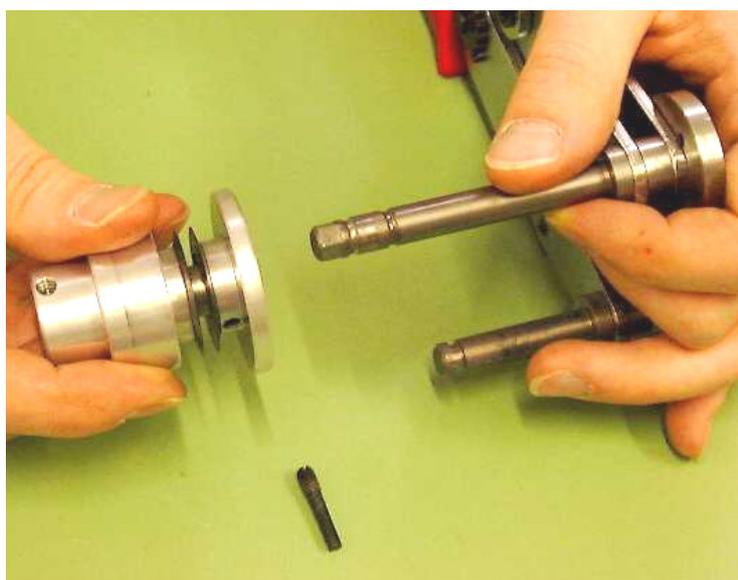
During assembly the tapered screw is fixed with care. The cutting weel must be free from play but easily turnable onto the axis!
