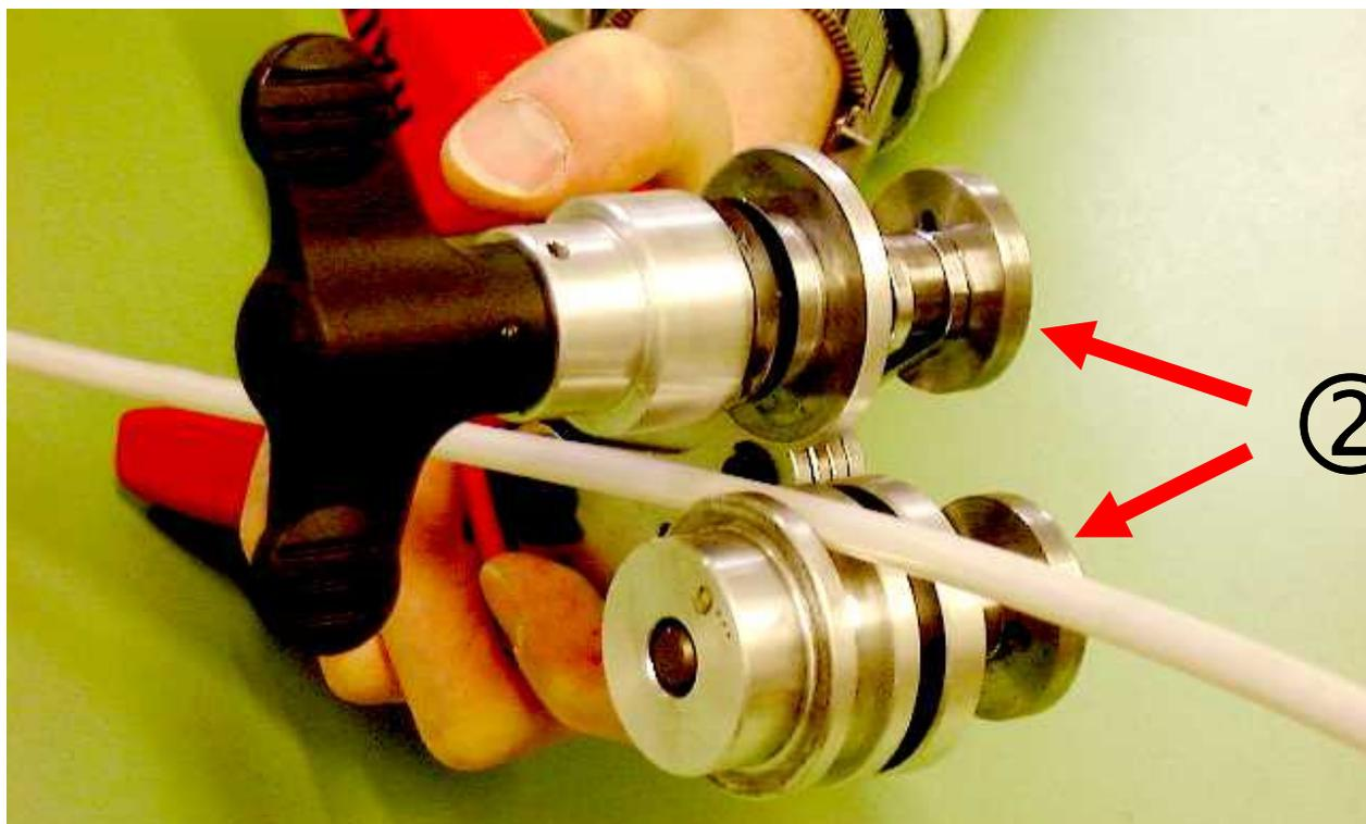
Close the tool slowly (1) until the guide axis roller touches the cutting axis roller (2). Simultaneously turn the butterfly handle backwards and forwards (3), to enable the knives to cut gently into the buffer tube. This prevents the thin knife blades from damage.
