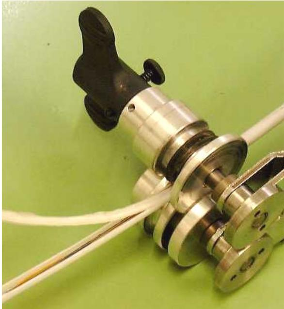
If problems occur, while using the tool, the RAUCUT II UNI can always be opened by pressing the small lever (arrow) between the two tool handles.
