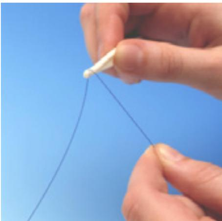
15. Lift the single fiber with help of the spatula; the white color ensures that the colors of the single fibers are clear visible. Select desired fiber(s) and break them in the slit on the bottom of the spatula or... (See point 16)
