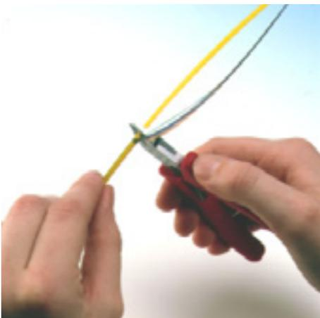
16. ... Lift out the single fiber or fiber bundle and use a side cutter to cut off the leftover insulation on both sides. Clean the fibers.
