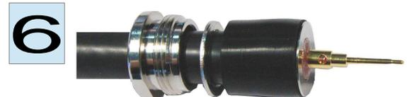
Attach inner pin to the inner conductor and solder carefully. Hint:
