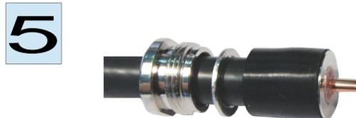
Remove the copper foil and the dielectric with a knife.
