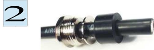
Move the nut, clamping ring and rubber washer over the cable tail. Hint: With a bit of Vaseline the rubber washer can be moved easily over the cable sheath.
