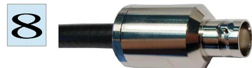
The prepared cable tail has to be inserted into the housing until stop. Tighten the clamping nut finger tight with two open-ended spanners 16 mm. A small split should remain visible between clamping nut and connector housing. Then the inner conductor has to be soldered to the center contact.
