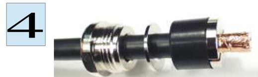
Bend copper braid upwards right-angled. Insert contact sleeve between copper foil and braid until stop. Cut off protruding braid. Move the rubber seal to the front, up to the contact sleeve.
