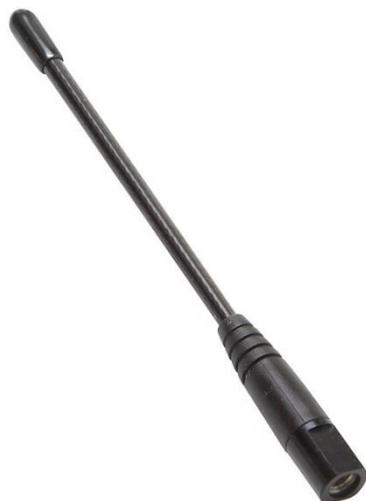
High quality flexible wire rod for 380-445 MHz. The antenna is normally used for Tetra, and is commonly used for Ambulances, Police cars, busses and other PMR applications. The rod fits with Smarteq antenna bases ANT, Base 1123, Base 128, Base 2500, MidiMag and MaxiMag.
