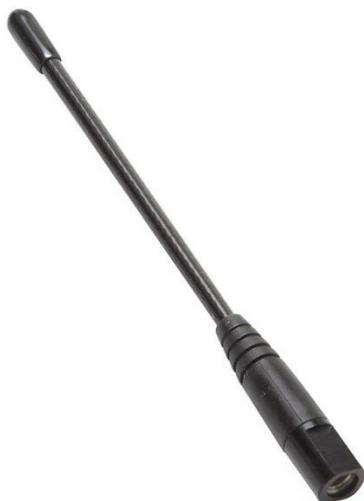
High quality flexible wire rod for 445-470 MHz. The rod is commonly used for Machine to Machine, and IoT applications over CDMA 450, ISM and Tetra. It's also used for Vehicles. The rods fits with Smarteq antenna bases ANT, Base 1123, Base 128, Base 2500, MidiMag and MaxiMag.
