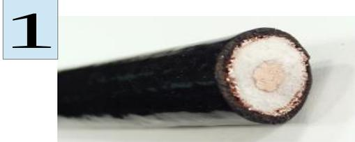
Cut off cable tail right-angled with a small metall saw. The inner conductor has to be kept absolutely round.
