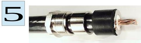
Remove the copper foil and the dielectric with a knife. The inner conductor must stay absolutely round. Remove burr from sharp edges.
