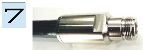
The prepared cable tail has to be inserted into the housing until stop. Tighten the clamping nut finger tight with two open-ended spanners 19 mm. A small split should remain visible between clamping nut and connector housing.
