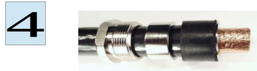
Bend copper braid upwards right-angled. Insert contact sleeve between copper foil and braid until stop. Cut off protruding braid. Move the rubber seal to the front, up to the contact sleeve.
