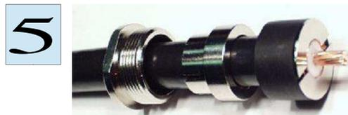
Remove the copper foil and the dielectric with a knife. The inner conductor must stay absolutely round. Remove burr from sharp edges.
