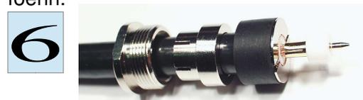
Move inner pin into the teflon-isolator. Subsequently, clip inner pin carefully onto the inner conductor. Hint: The inner conductor can be prepared with just a slim film of Vaseline, before attaching the inner pin. This improves the attenuation of intermodulation and prevents corrosion.
