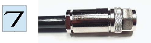
The prepared cable tail has to be inserted into the housing until stop. Tighten the clamping nut finger tight with two open-ended spanners 17/18 mm. A small split should remain visible between clamping nut and connector housing.
