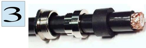
Remove 6 mm of the outer sheath with a knife.
