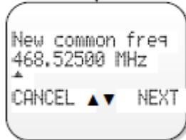
Increase or decrease the value of each digit by pressing ▲ or ▼. Move to the next digit by pressing NEXT. Repeat the procedure until the frequency is fully set.
