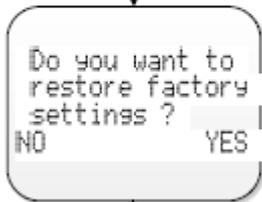
Press "YES" and the configuration will return to the same the radio modem was delivered with.
