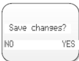
By choosing "YES" the configuration is saved into the non-volatile memory inside the radio modem.
