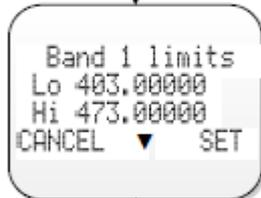
The limits of the Frequency Band 1 will be shown for informative purposes. Likewise the limits of Frequency Band 2 will be shown by pressing ▼. Press “SET” to activate the window for entering the frequency.
