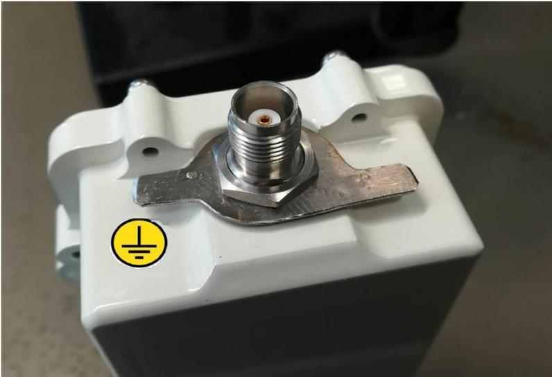
Besides the mains voltage safety, proper grounding is essential also for the error free operation of radio links and the protection against over-voltages and lightning. Although SATEL EASy-Proof incorporates a robust internal surge protection, the surge spikes and power transients caused by lightning, ESD or other electrical systems must be discharged to earth ground.
