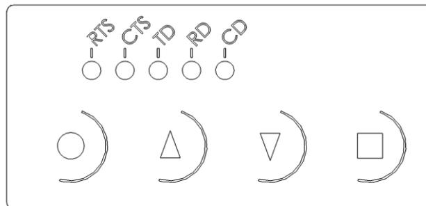
There are five (5) LED indicators on the front panel of the radio modem that indicate the status of the serial port and the radio interface:
