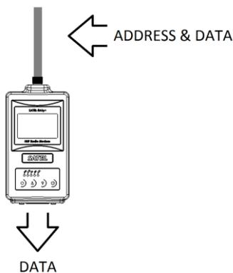
Reception addressing has been set ON and either the primary or secondary RX address of the radio modem is identical to the address of the received data packet.
