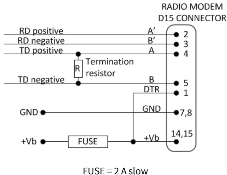
If the transmission lines are long the receiving end of the lines must be terminated using a separate termination resistor (typical values range from 100 -120 ohm depending on the characteristic impedance of the transmission line).
