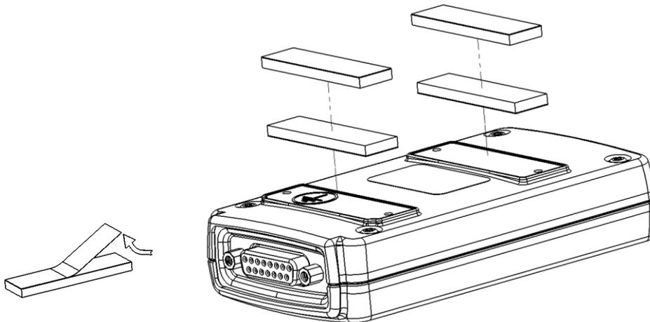
Figure 1.6 Velcro tape positions
