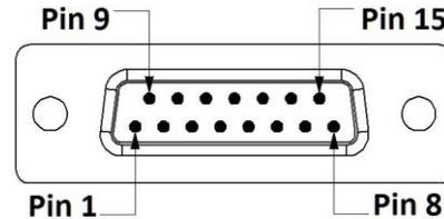
SATEL-EASy+ radio modems: 15-PIN FEMALE D CONNECTOR PINOUT
