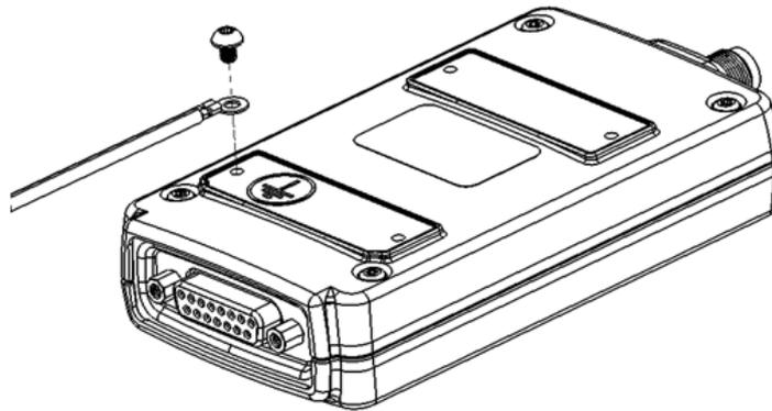
Figure 1.8 Grounding to the back of the housing
