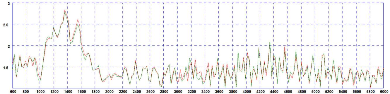
\*VSWR for elements assemblies 1 and 2 measured with 5m (16') of CS32 cable.
