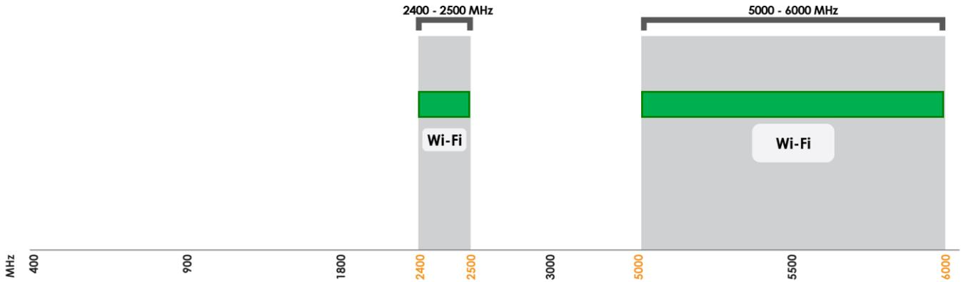
Indicates the Wi-Fi bands on which WLAN-61 works
