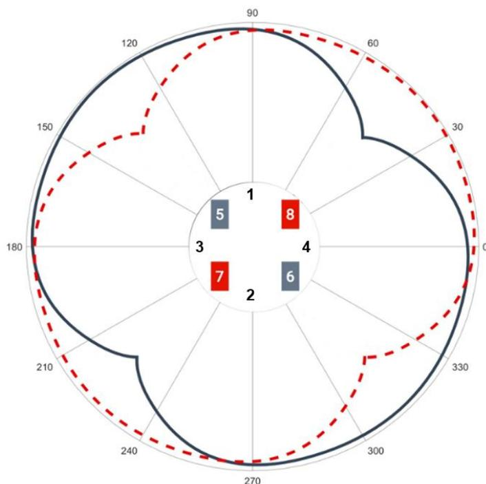
The overlay below details the connector positions and their connected Antenna radiation direction.
