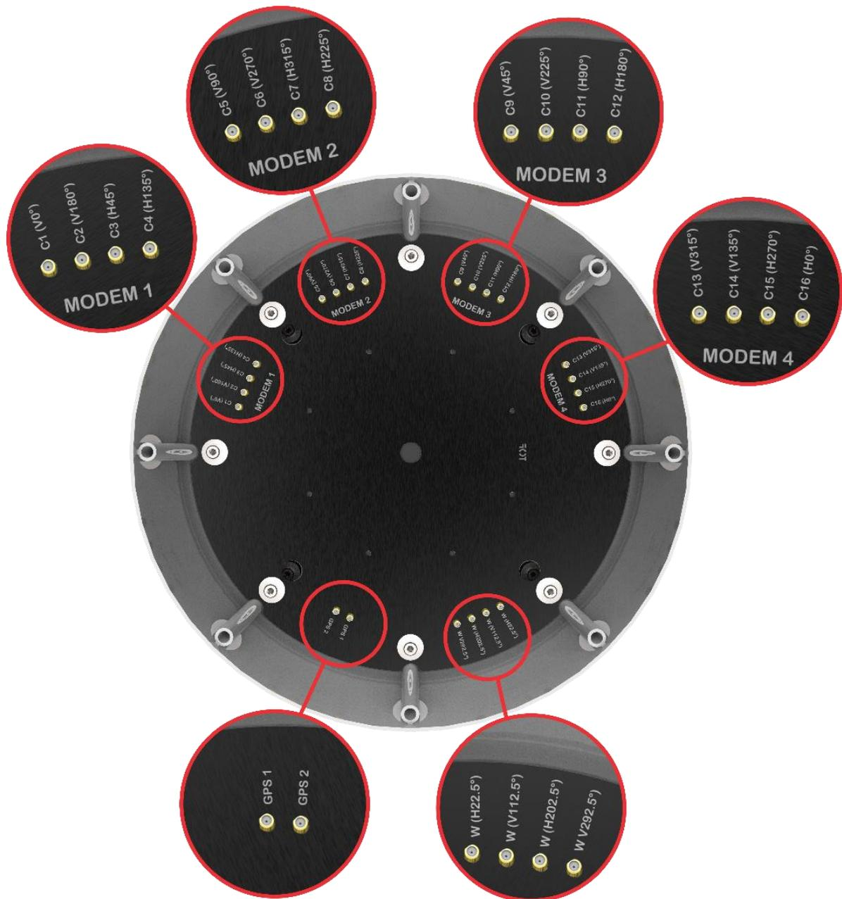
The overlay below details the connector positions and their connected Antenna radiation direction.
