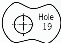
Mask panel area around hole position to protect paintwork and headliner. Drill a pilot hole, and then increase to 19mm (3/4"), ensuring that drill/ cutter bit does not contact headliner. Clean area around the hole, carefully removing all swarf.
