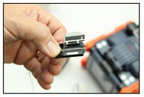
Hint: it is easier to load the fiber into the adapter if the fiber is curled in a downward direction from the fiber clamp.
