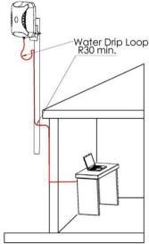
**Note:** The water drip loop is for preventing water from running down from the CPE along the cable into the house and possibly the PC.
