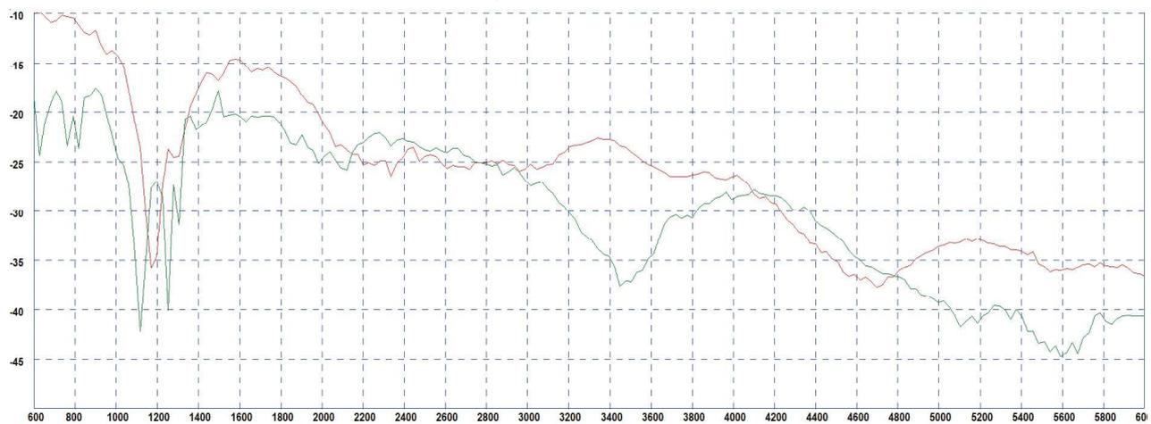
\*\*\*\*Red Plot = typical isolation adjacent elements, Green plot = typical isolation opposite elements measured in free space with 3m (10') of RG174 cable.
