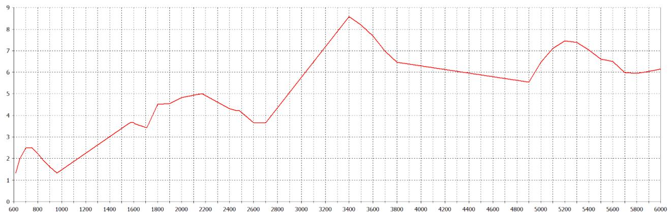
\* Swept peak gain simulated in CST Microwave Studio without cable loss.
