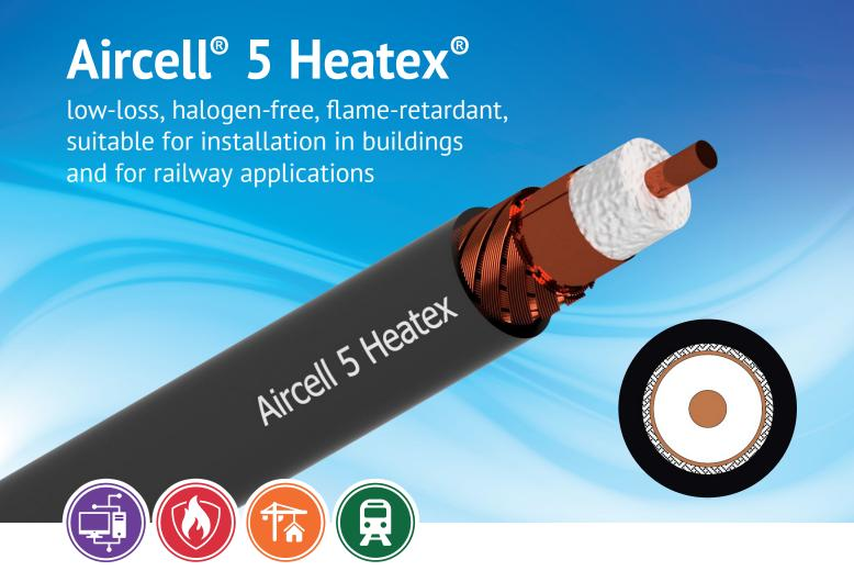
Aircell 5 Heatex is a flexible and thin coaxial cable with a 5 mm outer diameter designed for the frequency range from DC to 10 GHz. Its low-loss characteristics and compatibility with standard RG 58 connectors make it the top choice not only for Wireless LAN applications but also for general RF communications.
