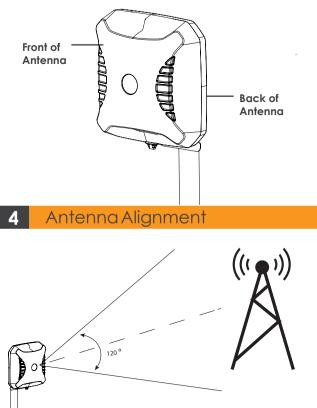
• To optimise the antenna alignment, rotate the antenna left and right in 15° increments until you get the best signal strength reading. Lock the antenna down at the position where you get the best signal strength.
