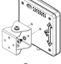
Mount bracket assembly to back of antenna as shown using screws and washers supplied.
