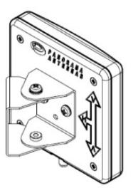
Secure to wall using 2 appropriate screws (not supplied).
