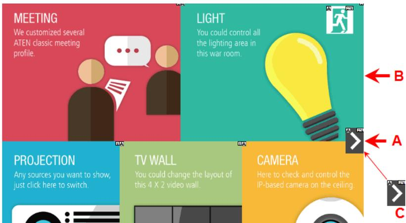
When the top button (A) is pressed, the lowest button (C) will execute the action.
