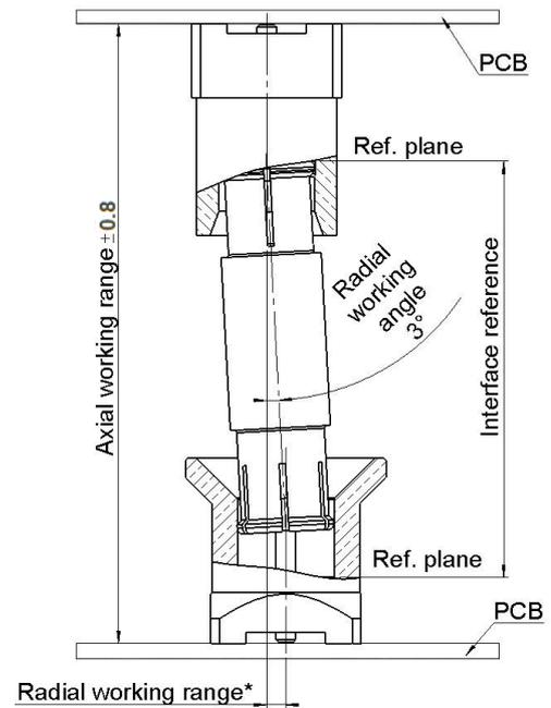
The connecting range represents the maximum misalignment during connection.
