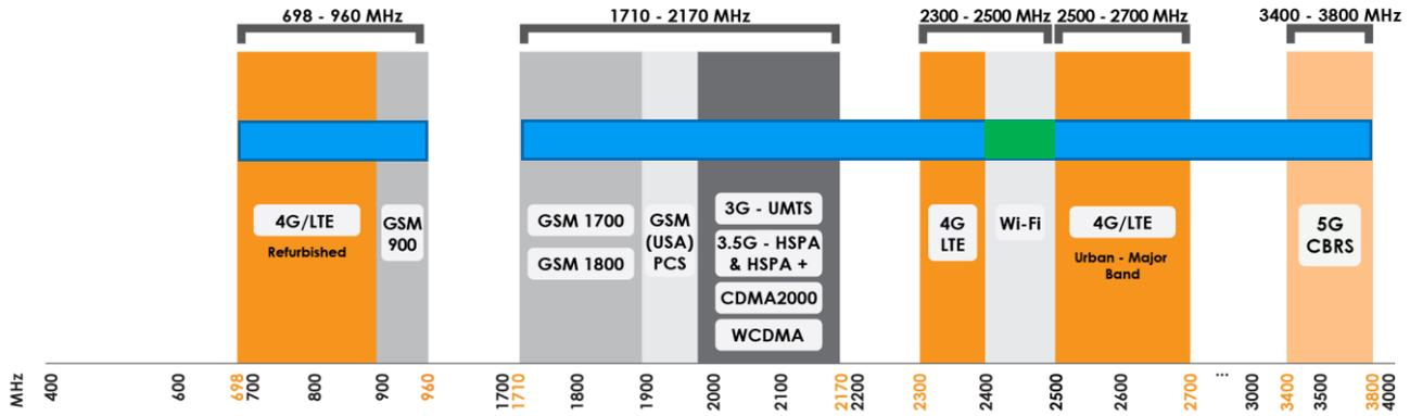
█ Indicates the LTE/5G bands on which OMNI-404 works     █ Indicates the WI-FI bands on which OMNI-404 works
