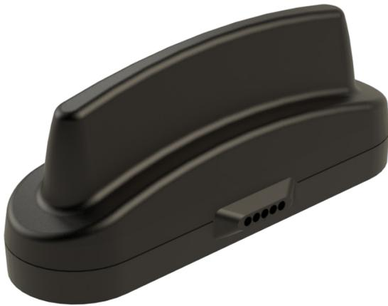
The LP[G]AMM-BC3G-26 range has been designed to provide MiMo Cellular / LTE antenna function for IOT and M2M applications. The compact, robust low-profile housing is weatherproof and contains two antenna elements with effective isolation and correlation covering all current global cellular and LTE bands in freq. range 698-960/1710-3800MHz.
