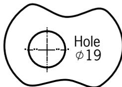
Mask panel area around hole position to protect paintwork and headliner. Drill a pilot hole, and then increase to 19mm (3/4"), ensuring that drill/cutter bit does not contact headliner. Clean area around the hole, carefully removing all swarf. Remove paint and primer from under panel surface to ensure adequate earth contact by washer and nut. Apply some petroleum jelly or paint around the hole to prevent corrosion.
