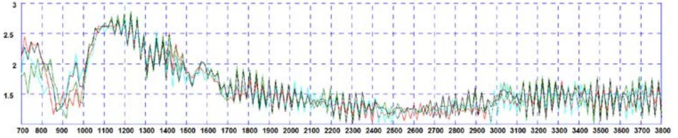
\* VSWR measured with 3m (10') of RG174 cable Green and Red Plots = Elements 1&2 in free space Black and Blue plots = Elements 1&2 on a 400x400mm ground plane
