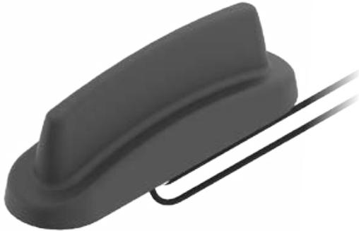
The LP[G]AM-BC3G-26 range has been designed to provide MiMo Cellular / LTE antenna function for IOT and M2M applications. The compact, robust low-profile housing is weatherproof and contains two antenna elements with effective isolation and correlation covering all current global cellular and LTE bands in freq. range 698-960/1710-3800MHz. The LG version includes an active GPS/GNSS/Galileo/Beidou antenna for applications which require position or timing function.
