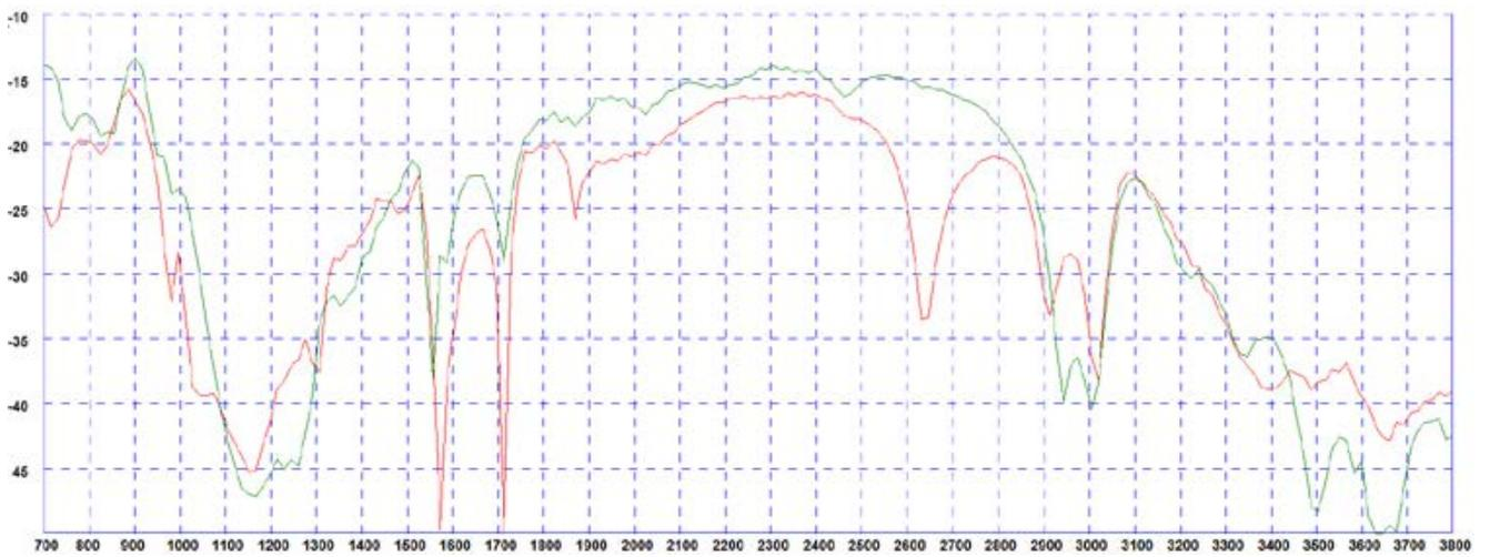
\*Isolation measured with 3m (10') of RG174 cable Red Plot = mounted on a 400x 400mm (1' 4" x 1'4") ground plane Green Plot = free space
