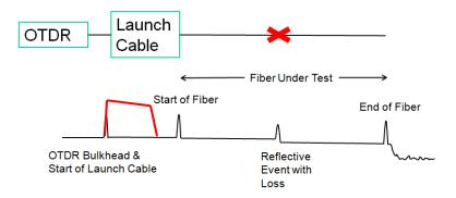
The deadzone of an OTDR is specified at the shortest pulse width. The IEC specification is a pulse width of 5ns while measuring an event of -45dBm reflectivity. More reflective events will cause a longer deadzone. It is imperative that all connectors are cleaned and inspected so as to avoid contaminated and or damaged connectors that will be more reflective and cause a longer deadzone.
