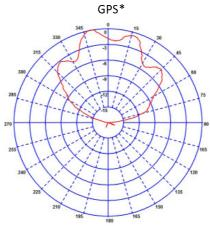
\*measured on a 160x160mm ground place
