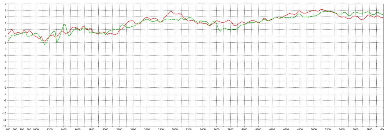
\*Peak Gain elements 1&2 measured in free space with 0.5m (1.6') of RG174 cable
