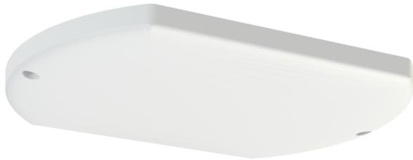
The CMSLP-038-4 range has been designed to provide SiSo UHF/3G/4G & 3.8GHz 5G coverage for DAS networks in an ultra low profile package. The compact, robust low-profile housing contains a highly efficient antenna element covering 380-520/617-960/1710-3800MHz.
